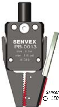
3 Sprue gripper is Closed; and missing the sprue. The red spring loaded lever arm remains in its open position although the gripper is closed.
