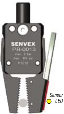
2 Sprue gripper is Closed; gripping the sprue. Pressure from the sprue deflects the red spring loaded lever arm into the gripper finger. The close proximity of the lever arm to the sensor closes the circuit, illuminates the LED, and indicates that the sprue is gripped.
